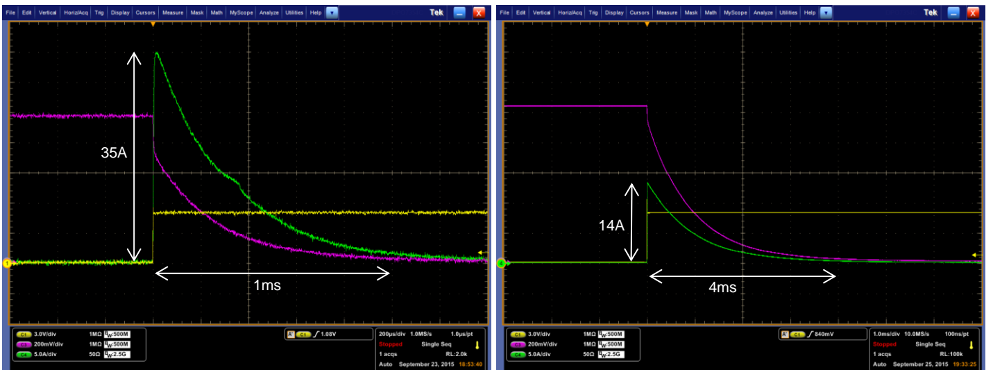
Figure 8 Sub-zero temperature measurements (approx. T_a=-20^\circ\text{C} ). Left curves = 35A peak current discharge through DMN3027LFG channel resistance only (200μs/div) Right curves = 14A peak current discharge through DMN3027LFG and 50mΩ series resistor (1ms/div)
