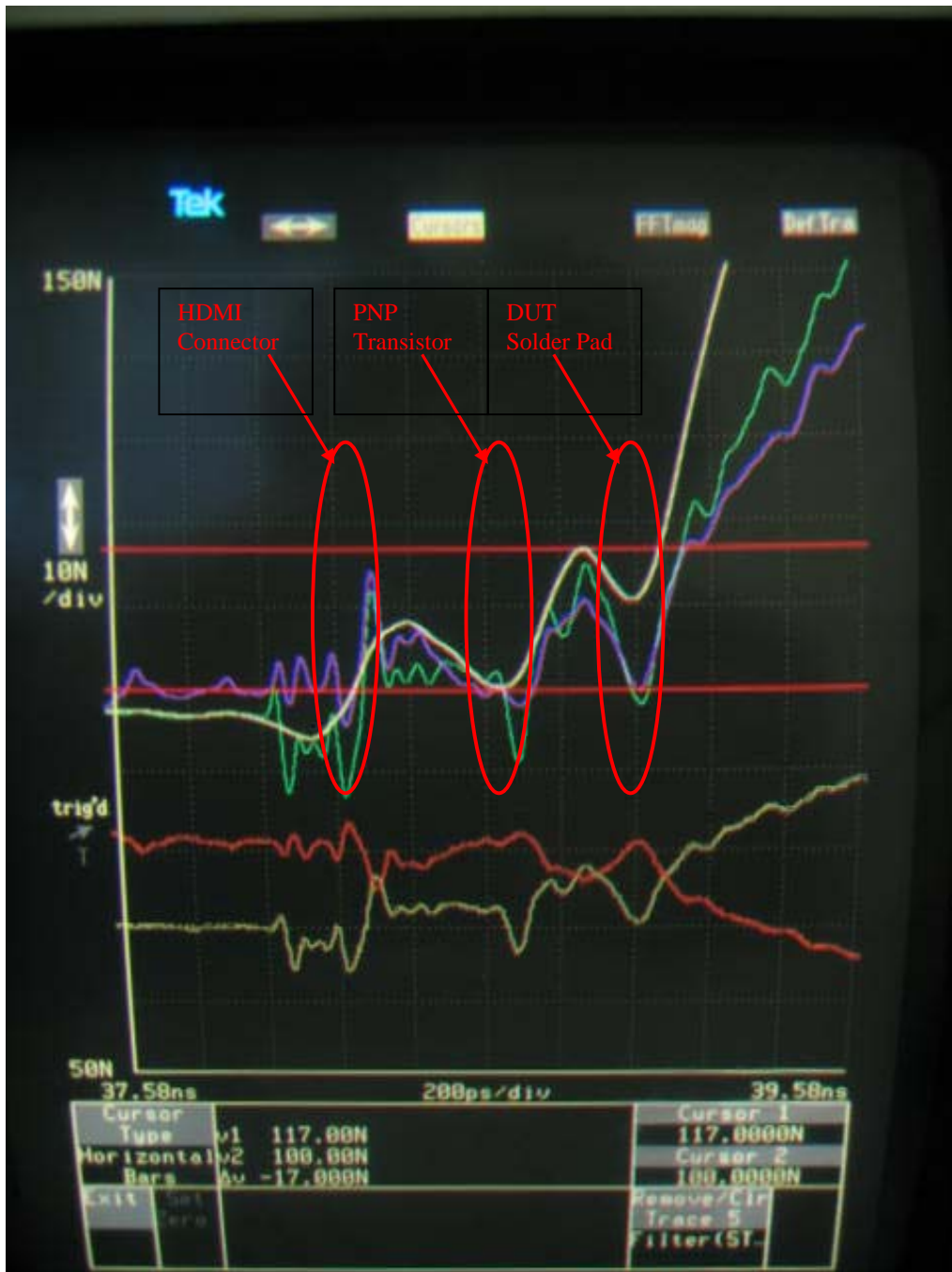
Figure 9: TDR Plot at CLK with pnp Transistors
