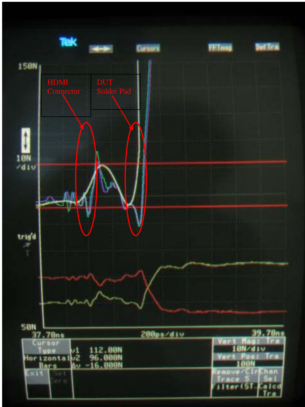
Figure 8: TDR Plot at CLK without pnp Transistors
