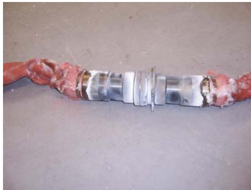
High temperature connector after 30 minutes in 800°C oven
