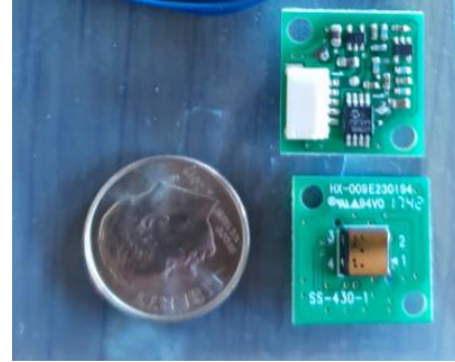
Sensor mounting surface Component mounting surface
