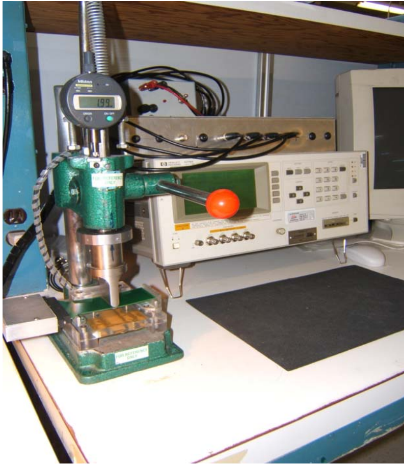
Figure 14 Flex Test Fixture W/CPU for Data Storage
